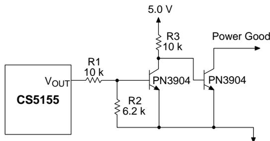
**Figure 17. Implementing Power Good with the CS5155**
