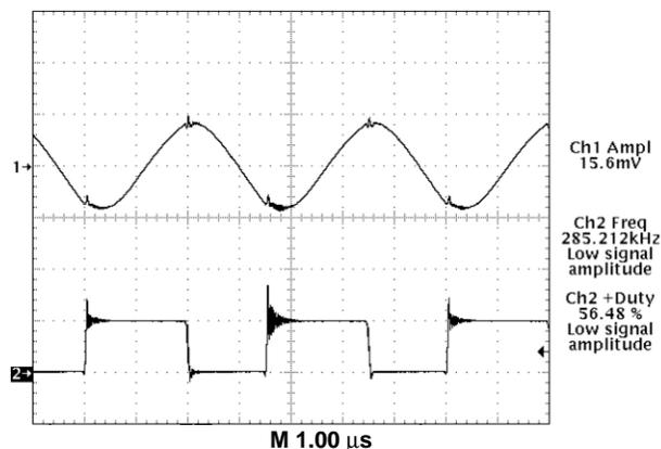
Trace 1— Regulator Output Voltage (10 mV/div.)
