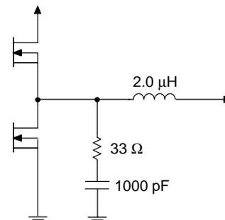
Figure 20. Filter Components
