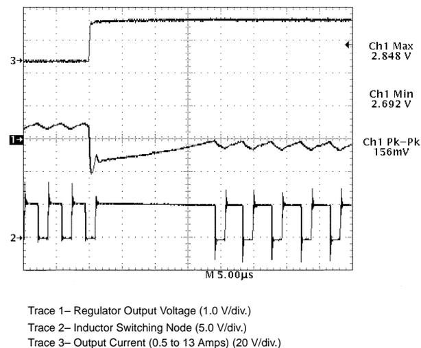
**Figure 10. CS5155 Demonstration Board Response to
